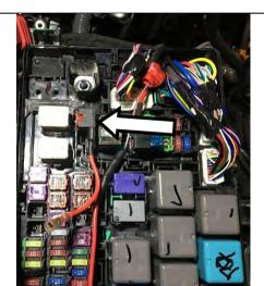
34. Find the fuse tap included in the harness bag and plug the removed fuse into the lower slot of the tap.
