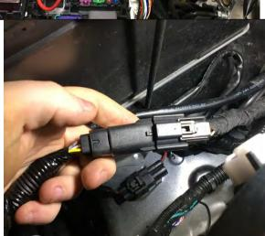
43. Disconnect the 6-pin connector from the back of the headlight on the left side of the vehicle. Plug this connector into the corresponding side of the harness headlight connectors.
