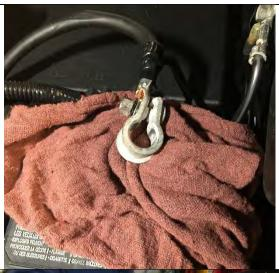
Disconnect the battery's main ground from the battery and push the cable to the side. A rag or other cover can be used to ensure the wire does not touch the battery terminal.
