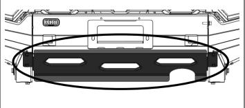
Assemble stone shield with four flanged M8x1.25x25mm bolts (two per side). Torque to specification.
