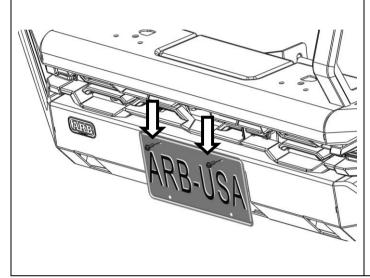
77. If fitting a licence plate, use two M6x1.0x16mm button heads, 12mm M6 washers, and M6 flange nuts to attach the plate.
