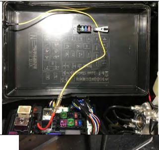
42. Connect the harness side of the bullet connector to the fused side and reinstall the fuse box lid.
