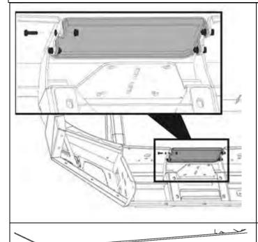
48. If not fitting a winch, assemble the winch cover panel to the bar using four M6x1.0x20mm hex bolts, 12mm flat washers, and flanged M6 nuts.
