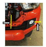
22. Cut the corners off as indicated in the picture using an oscillating multi-tool.
