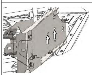
Once happy with the position of the bar and all fasteners are correctly torqued, using the existing 2 holes in the mount as a guide, drill through using a 10mm drill bit and secure using two flanged M10x1.5x30mm bolts and M10x1.5 flange nuts, tighten to specification.
