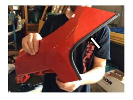
28. After removing the cut bumper end, remove masking tape and deburr all edges with file or sandpaper.
