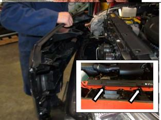
If fitted, remove licence plate from bumper.Remove the two top screws on the grille.
