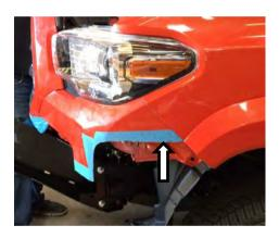
26. Using the refitted cut bumper end as a guide mark the bumper retaining bracket.
