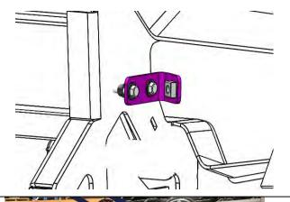
55. Assemble two M6 (2.6-3.5mm) caged nuts into both fog cluster mounting brackets.
