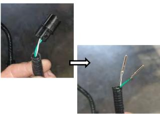
45. If the vehicle comes with OE fog lights, cut the OE connector off the loom and fit the Deutsch connectors as shown. If there were no OE fog lights on the vehicle, use ARB harness 3500520.
