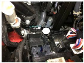
37. Cut a matching slot into the fuse box directly next to the latch on the right side.
