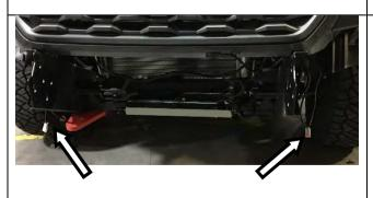
47. Feed the loom down behind the vehicle grille and route across the chassis mount brackets as shown.
