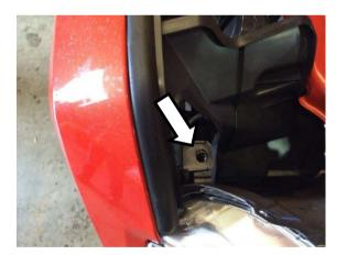
3. Remove grille from vehicle by removing the clip shown near the head light on both sides and then release lower grille tabs by pushing up as shown below.
