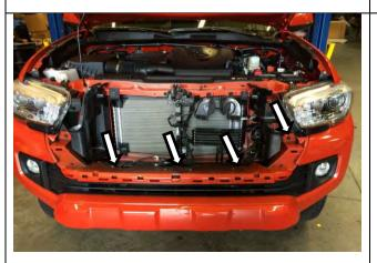
Remove the bumper, by releasing the clips along the top return and below the head light.
