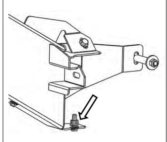
Leave bottom M12 bolt from step 14 loose enough to rotate the wing panel bracket if needed.
