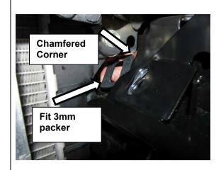
13. Fit two 3mm packers as shown into the upper mount reinforcement. Fit flanged M12x1.25x35 bolts and flanged M12x1.25 nut. Leave finger tight.
