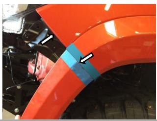
24. Mark the fender flare as shown. Use masking tape to protect the fender flare and using the fender edge as a guide, mark the fender flare. Repeat for other side.
