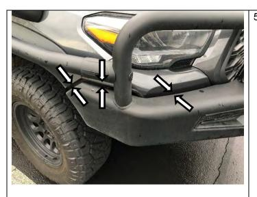
Align bull bar so there is a 15-18mm gap from top of wings to underside of flares and an even 10mm minimum gap to vehicle including periphery under headlights, and then tighten all bolts.
