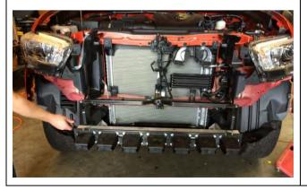
8. Remove the plastic from the crash beam and unclip the side brackets (from underneath).
