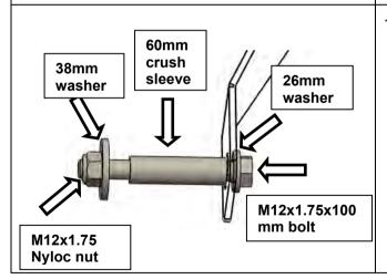
15. Use M12x1.75x100mm bolt, 26mm washer, 38mm (1.5") washer, 60mm crush tube, and Nyloc nut to fasten the rear of the tensioning bracket.
