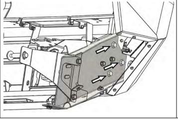
58. Loosely fasten bar to chassis mount brackets using six flanged M12x1.25x35mm bolts and six M12 flange nuts.
