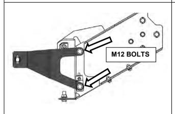
14. Fit tension brackets to each side of vehicle. Affix using two flanged M12x1.25x35mm bolts and flanged M12x1.25 nuts. Place the wing panel bracket under the lower flanged bolt as shown below.
