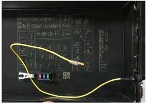
41. Insert bullet connector through grommet in fuse box lid until the sheathing is inside the grommet. Wire can be routed underneath the fuse puller.
