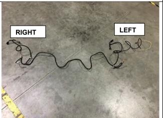
38. Identify the left and right side of harness 6821471. The left side of the vehicle will have the yellow wire with the bullet connector which will go to the fuse box.
