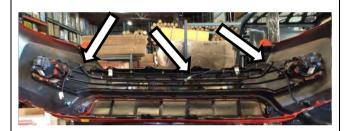
17. If fog lamps are fitted to the bumper remove harness and set aside. This will be reused later.
