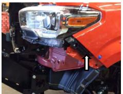
25. Using masking tape, mask up the bumper end and retaining bracket across the centre of the part.
