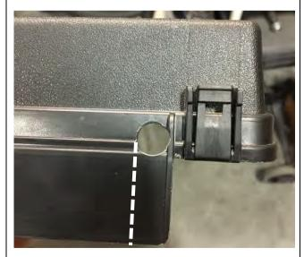
35. Drill a ø10mm hole in the right side of the fuse box cover right next to the edge as shown. Trim parallel to the edge, straight down.
