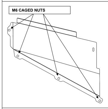
Fit four M6 (0.7-1.6mm) caged nuts to the inside of the flanges on the wing under panel, RH & LH.
