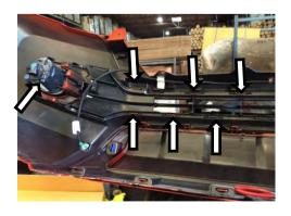
19. To make the bumper cut easier remove the fog lamp (if fitted) and the plastic grill insert in the bumper by depressing these tabs around the edge.
