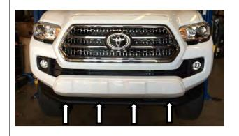
5. Remove the clips and screws along the bottom edge of the bumper.
