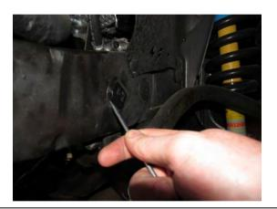
11. Remove plastic plugs in chassis holes in 4 places, inside and outside chassis in the area shown.
