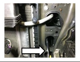
40. Route the bullet connector and headlight connectors on the left side of the vehicle through the hole shown.
