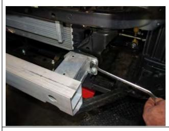
9. Remove and discard crash beam, retain nuts for re-fitment later.
