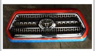
18. Mark out the centre grill section. Place marking tape along the bottom edge and with non-permanent marker, mark a line 18mm from the bottom lip.
