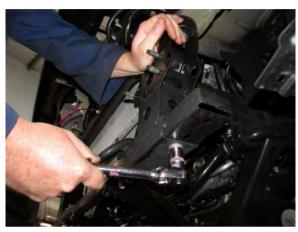
10. Remove lower bolts on cross member and remove cross member extensions both sides as shown and discard.
