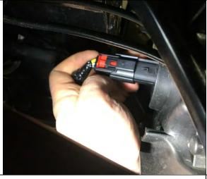
14. Insert other side of the 6-pin connector into the back of the headlight.
