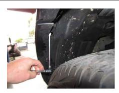
6. Remove the two front wheel arch bolts. Pull bumper ends out and away from vehicle to release them from clips. You will also need to unclip the wheel arch flare. Remove bumper and place on work stand front face up.
