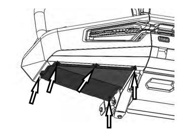
Assemble wing under panel using ten flanged M6x1.0x25mm bolts (5 per side). Torque to specification.
