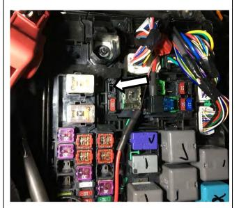
33. Remove the fuse panel cover located on the left side of the vehicle's engine bay.
