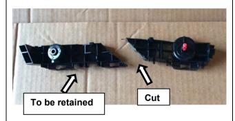
27. Using an oscillating multi-tool carefully cut the bumper retaining brackets along marked lines.
