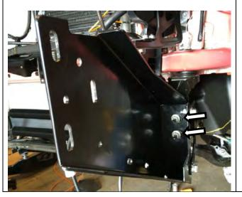
12. Fit the chassis mount bracket assembly to the front of the vehicle using the six M10 studs to locate on.
